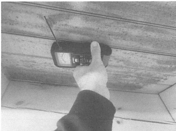
A9 (Moisture readings taken from the affected ceiling in Stephanie's office were not elevated at the time of the inspection.)
