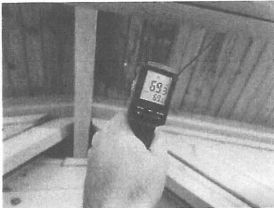
A7 (Surface temperatures taken from affected and unaffected ceiling materials matched at the time of the inspection.)
