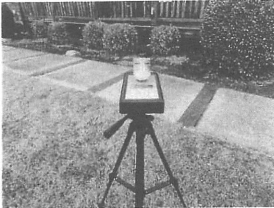
A1 (The sampling pump was calibrated onsite for accurate testing. An air sample was taken outside and was sent to IMS labs for analysis.)
