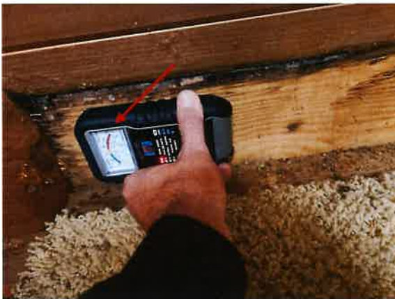
A12 (Moisture readings taken from the affected wood were elevated at the time of the inspection.)
